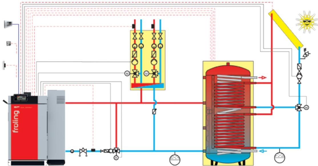
SP Dual compact with layered tank and hot water heat pump
